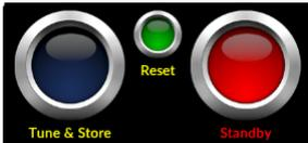
The power amplifier is in standby mode and the tuner is inactive (the **Tune** button is dark blue).
