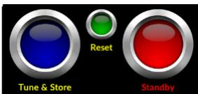
There is a carrier signal at the input of the power amplifier. The antenna tuner is ready for tuning (the **Tune** button becomes slightly brighter).
