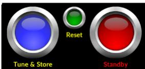
The internal antenna tuner is in the tuning process (the **Tune** button lights up light blue).
